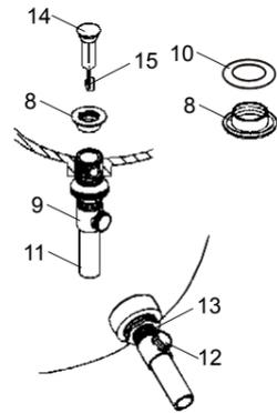
Place stopper(14) into drain body aligning the flat side of stopper hole(15) with the drain lever hole.
