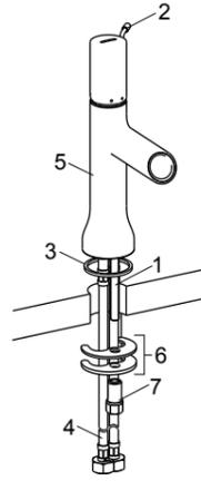
Attach the hoses to water supplies. When facing the front of the faucet, the left hose connects to hot water, the right hose with "COLD" label connects to cold water.
