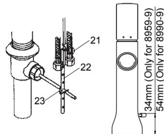
Push the ball lever down into the open position. Tighten thumb screw.
